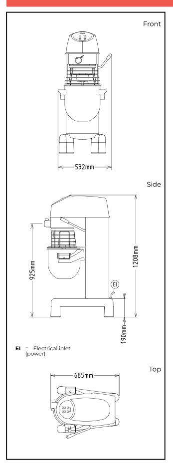
Electric Supply voltage: 200-240 V/1N ph/50/60 Hz Electrical power, max: 1.1 kW **Total Watts:** 1.1 kW Capacity: Performance (up to): 7 kg/Cycle Capacity: 30 litres Key Information: External dimensions, Width: 532 mm External dimensions, 685 mm Depth: External dimensions, Height: 1208 mm **Shipping weight:** 114 kg **Cold water paste:** 7 kg with Spiral hook 50 with Whisk Egg whites:
